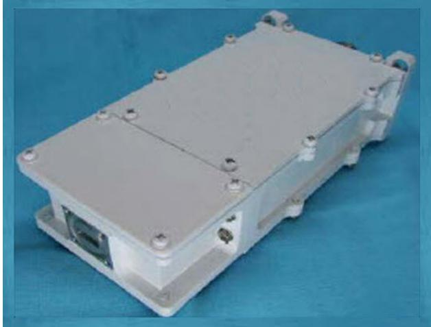
RADITEK's announces a new LNB. Phase locked LO, Ka band, (20.2-21.2GHz). Noise figure 1.7dB, 60 dB gain. Operates from 18 to 24V @ 400mA max., WR42 interface, type N IF out, 10MHz reference in, on DC bias line/IF port. 45 dB image rejection and 15dBm P1dB. If frequency 1-2GHz. Operates to 10,000 feet ASL.
